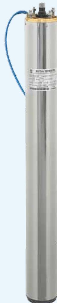
The internal cooling is guaranteed by non-toxic dielectric fluid conforming to the standards of the Italian and European Pharmacopea and those of the Food and Drug Administration of United States. Motor sealing is performed by three seal levels. Widely sized rubber expanding diaphragm to allow the equalization between the motor internal and external pressure without exchange of liquids. Bidirectional rotation.
